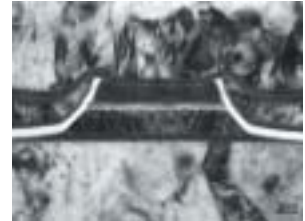
A TMR head (Tunneling-MR head) through an electron microscope
