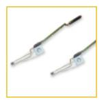
Product Overview ► The main products in this sector are magnetic recording heads used in HDDs. Magnetic recording heads read signals stored on disks using magneto-resistive elements. At present, GMR (giant magneto-resistive) heads are the mainstream in the HDD head market. These heads boast an extremely high magneto-resistive effect, greater than that of MR heads.
