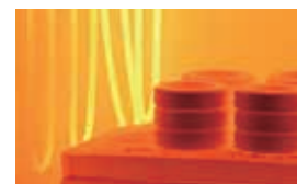
Sintering technology Sintering to solidify and harden with precision control of temperature and atmosphere (gas components in the furnace).
