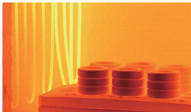
Sintering process of ferrite and temperature control
