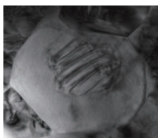
Core (center) and shell (surrounding part) structure of dielectric ceramics particles
