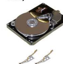
The internal structure of an HDD and magnetic heads
