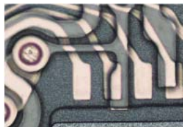
Multiple layer circuits by additive deposition
