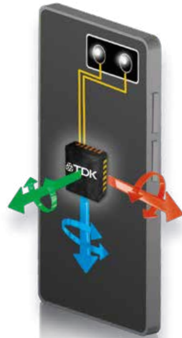
▲ICM-42600: World's first 6-axis MEMS Motion Sensor supporting dual-camera with dual-OIS image stabilization
