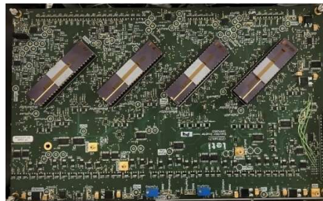
AI circuit board equipped with four ceramic packages
