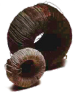
A coil that uses a ferrite core
