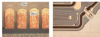
High density, thin micro coil by additive deposition
