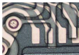
Multiple layer circuits by additive deposition
