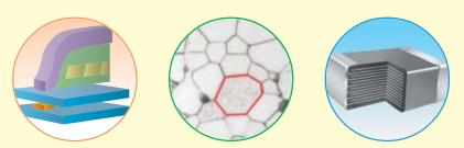
**GMR Head:** Pictured is a cross section of a GMR head for a hard disk. The spin valve of GMR heads, which is the part that actually retrieves data from the hard disk, showcases the sophistication of TDK's ultraprecise process, control and materials technologies. This microscopic element is fabricated by stacking many layers of film no thicker than a few nanometers on top of one another. And, incredibly, GMR heads float a mere 10 or so nanometers above a hard disk as it spins at high speed.
