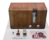
A super heterodyne-type radio receiver, and ferrite cores for IF transformers (foreground)
