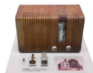
A super heterodyne-type radio receiver, and ferrite cores for IF transformers (foreground)
