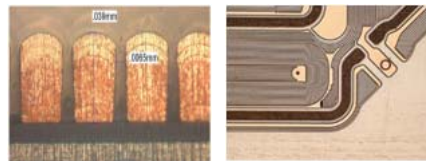
High density, thin micro coil by additive deposition
