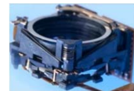
SMA (Shape Memory Alloy) Optical Image Stabilizer
